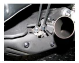
Now remove the oxygen sensor on the right side of the cat. Locate the oxygen sensor plug, (behind right side cover), and unplug it. Get some slack in the cable and twist it counterclockwise to avoid kinking it when you unscrew the plug.
