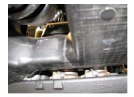
Loosen the clamps on the front header pipes securing them to the catalytic converter. Make sure there are no items you've inadvertently missed or ignored, and slide the cat off the front header pipes and out of the way. Now is also a good time to remove all the mounting brackets that held the cat on the frame. Also remove the clamping collars and packing gaskets from the rear header tubes on the cat.
