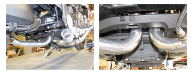
Remember to install the oxygen sensor in the right pipe. This is more easily done by holding the sensor and twisting the pipe onto it instead of twisting the sensor into the pipe. This will prevent excessive twisting of the wires. You can do the final tightening of the sensor once the assembly is tightened up on the bike. Re-connect the sensor plug and replace the boot.
