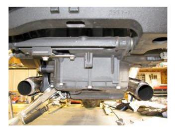
Now you will want to loosen the clamp bolt on the front header pipe cross over tube. Just a few turns will do it, you only need enough to let the pipes flex a bit.
