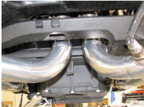
Remember to install the oxygen sensor in the right pipe. This is more easily done by holding the sensor and twisting the pipe onto it instead of twisting the sensor into the pipe. This will prevent excessive twisting of the wires. You can do the final tightening of the sensor once the assembly is tightened up on the bike. Re-connect the sensor plug and replace the boot.
