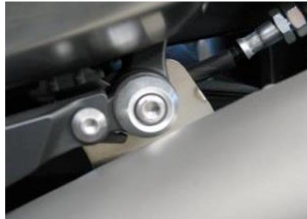
In order to remove the catalytic converter, first loosen the front header pipe. Only loosen the flange bolts enough to disconnect the cat from the rear header pipes. Use the 8mm X 3/8 ball driver for this. Just insert it between the radiators and into the front header pipe socket bolt.
