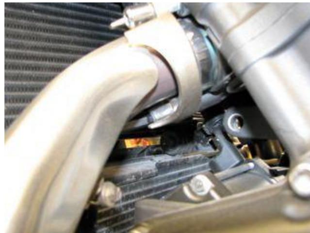
Next, remove the EXUP cables from the right side of the cat box. Secure them out of the way.
